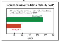
Idemitsu ATF maintains an optimum friction ratio longer than ordinary ATF brands
